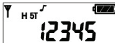
(Figure 8-4) Display shown on the RX Radio when transmitting with (Repeater) + Destination + RADIO ID
